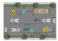
d) The Alma Street – Malakoff Street to Kains Street road section is greater than 8.0m measured at 10.5m in width with no parking restrictions on both sides. Signs and markings for the road section will be completed as depicted to the right.
