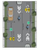
c) The Malakoff Street -Balaclava Street to Alma Street road section is less than 8.0m in width with no parking anytime restriction on the south side. Signs and markings for the road section will be completed as depicted to the right.
